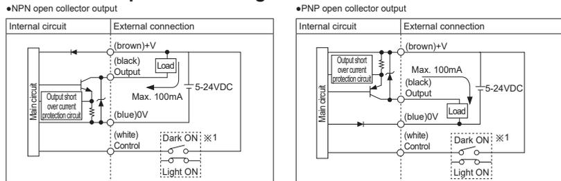
※1: Operation mode selection: Connect (white)Control cable (terminal) into terminal (brown)+V to operate Light ON mode. Dark ON mode is available with disconnection status.
